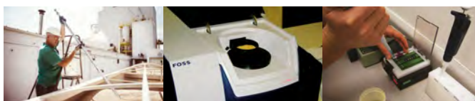
Bulk ingredients are sampled across the depth and length of the load and tested for macronutrients and mycotoxins
